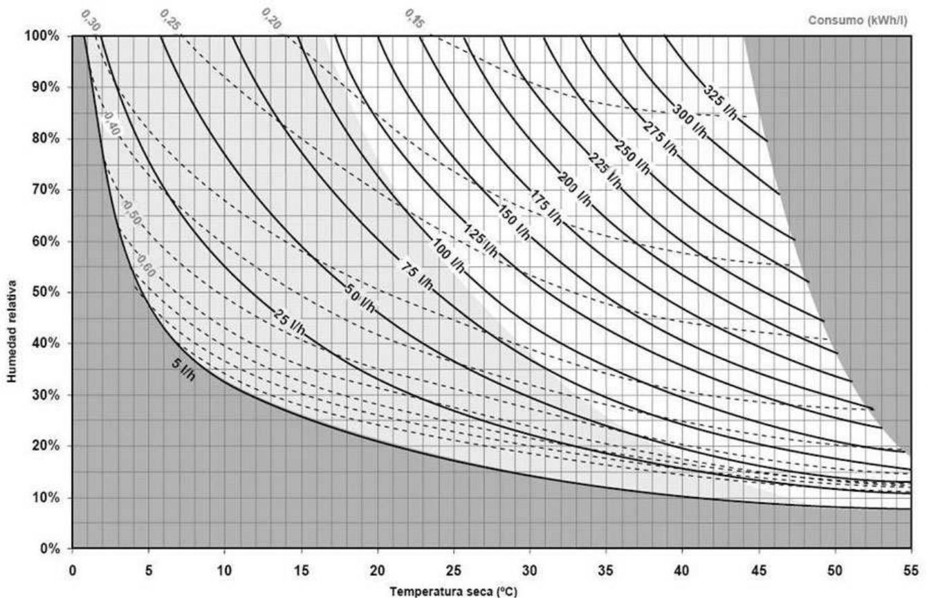
*Production and energetic cost according to the temperature (°C) and environment Relative Humidity for a 15000 m<sup>3</sup>/h machine*
