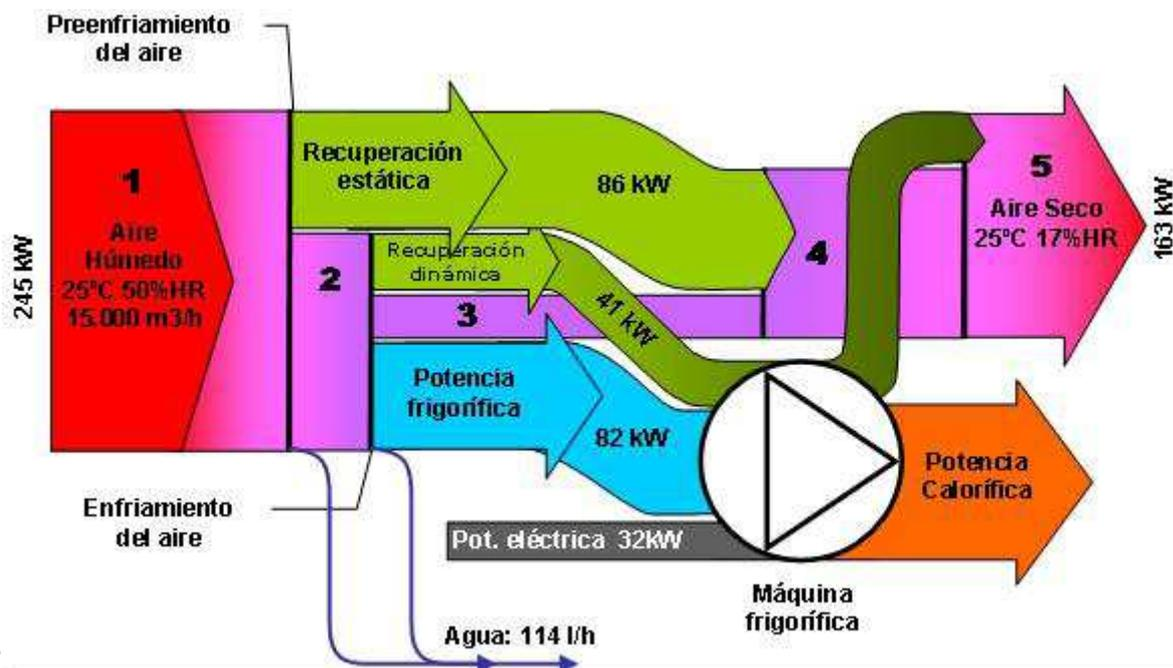
Enthalpy flows in the water producing machine for 25°C 50%HR environmental (source: Own elaboration).
